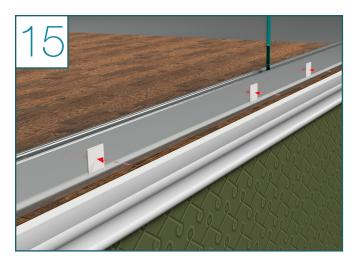
• Using the table below, stick the provided 2" adhesive pads to each base rail section using the table below
