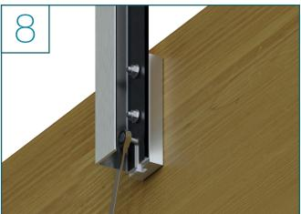
Once the post is fully seated in place, use the wrench to reach up through the bottom of the post and fully fasten the hex head lag
