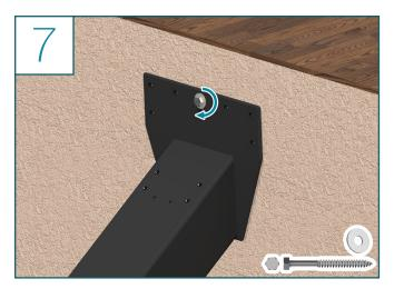
Fasten the <sup>1</sup>/<sub>2</sub>" x 3<sup>1</sup>/<sub>2</sub>" Hex Lag through the middle slotted hole in the header plate to hold the stringer in place
