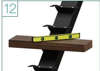
Ensure the tread is level on the tread bracket both front to back and left to right
