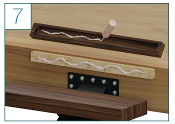
• Apply wood glue to both the Mounting Block and the inside cavity of the Nosing
