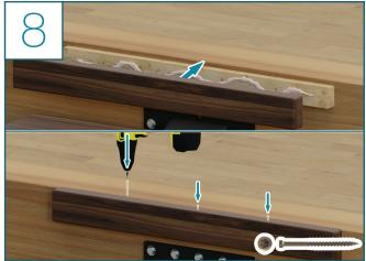
• Press the nosing firmly into place and use the T-10 bit to fasten #8 x 2" trim screws, holding the nosing cover in place
