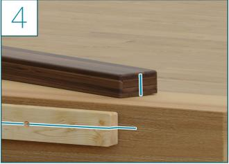
• Align the mounting block center line with the center line mark you drew in the previous step
