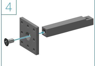
Using the <sup>1</sup>/<sub>4</sub>" - 20 x <sup>1</sup>/<sub>2</sub>" screw, attach the mounting plate to the base stem
