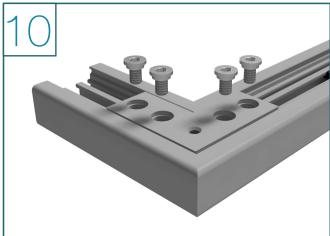
• If you have mitered corners, install the corner brackets with the provided bolts
