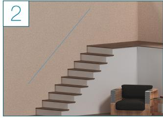
• Snap a chalk line to mark diagonally between the 2 marks (a laser level would work as well)
