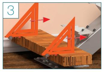
Slide both jigs on to the first tread so that the adjustment block rests up against the nose of the tread
