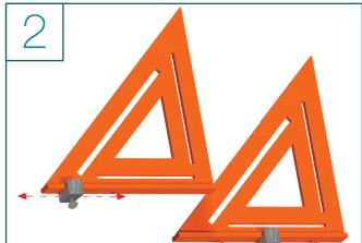
• Set the adjustment block to that dimension on both jigs
