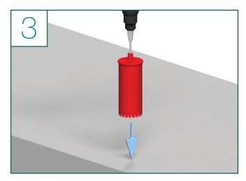
Use a 3" Concrete Core Saw to cut enough space for the post to sit in
