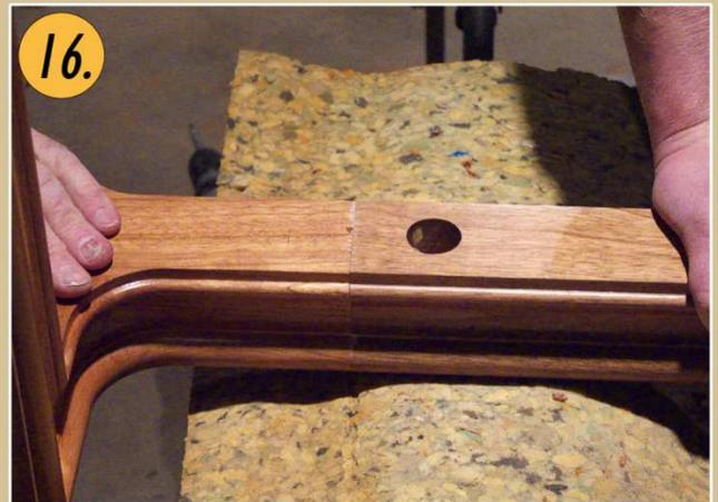
Once the glue is applied, fasten the nut to 80%, make sure everything is lined up, then tighten nut 100%.
