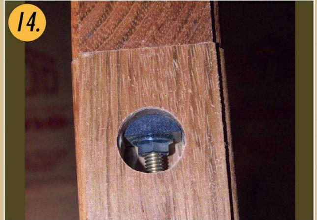
Using the wrench on the other end of the RAIL BOLT WRENCH, tighten the nut to 80%.
