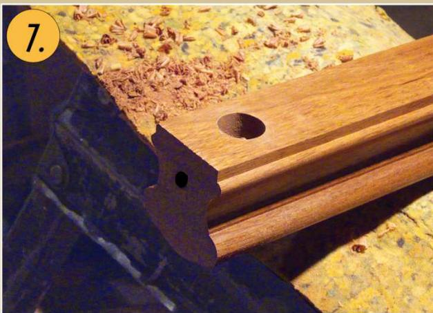
**7.** This is how your handrail should look after drilling holes from steps 5 & 6.
