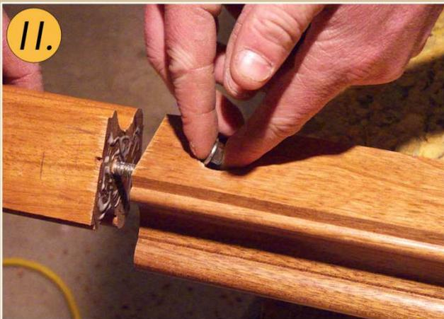
Insert metal nut into the 1" hole, and fasten to the machine end of the RAIL BOLT. Image shows doing this with fingers. We Recommend...
