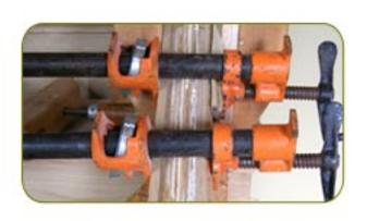
Begin to add clamps working from the center of the bend outward. You may find you have to loosen some clamps and re-tighten them. Look for consistent and even glue squeeze out along the top of the handrail. Any area that has a crack or uneven glue squeeze-out will need additional clamps. As a general rule, apply a clamp every six inches.
