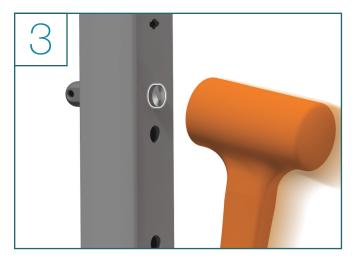
Using a rubber mallet and wood driver, drive the steel plug into the ½" hole
